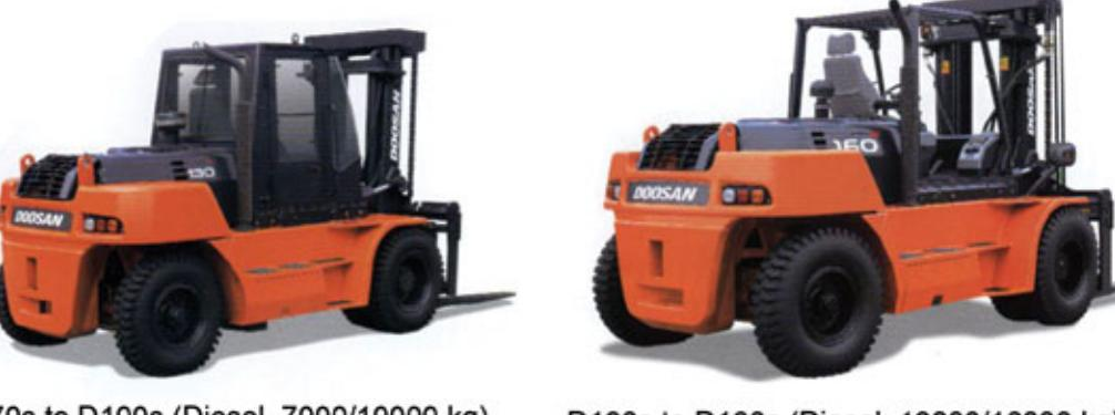
D70s to D100s (Diesel, 7000/10000 kg)    D130s to D160s (Diesel, 13000/16000 kg)
